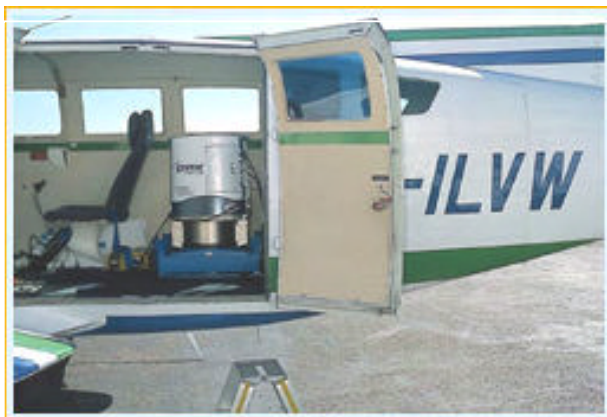
Figure 3. Installation of the DMC in the ILV aircraft
