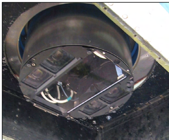
Figure 4. View from bottom to the DMC camera module with the separate objectives
